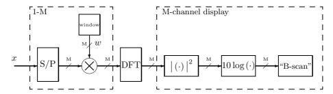
The following steps are performed: blocking up the time series/serial-to-parallell (S/P), windowing each block (multiplication by  $\{w_k\}_{k=0}^{M-1}$ ), computing the discrete fourier transform of the windowed block (DFT), taking the modulus square ( $|\cdot|$ ) or energy) and finally express the result in decibels ( $10 \log_{10}(\cdot)$ ) or dB).
