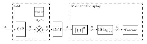
The following steps are performed: blocking up the time series/serial-to-parallell (S/P), windowing each block (multiplication by  $\{w_k\}_{k=0}^{M-1}$ ), computing the discrete fourier transform of the windowed block (DFT), taking the modulus square ( $|(\cdot)|^2$  or energy) and finally express the result in decibels ( $10 \log_{10}(\cdot)$  or dB).
